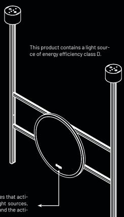
Control system with three touch switches that activate the switching on and off of the light sources, the selection of the color temperature and the activation of the anti-fog system.
